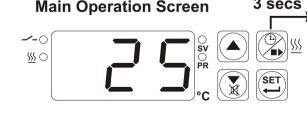
In main operation screen, If cooking button is pressed for 3 seconds, then cooking time (Timer) is started and cooking time active led becomes active. While cooking time (Timer) continues if cooking button is pressed for 3 seconds, cooking time (Timer) is finished and cooking time active led lights off. If button protection parameter P = 4 cooking time (Timer) ON/OFF operation is performed when button is pressed.
