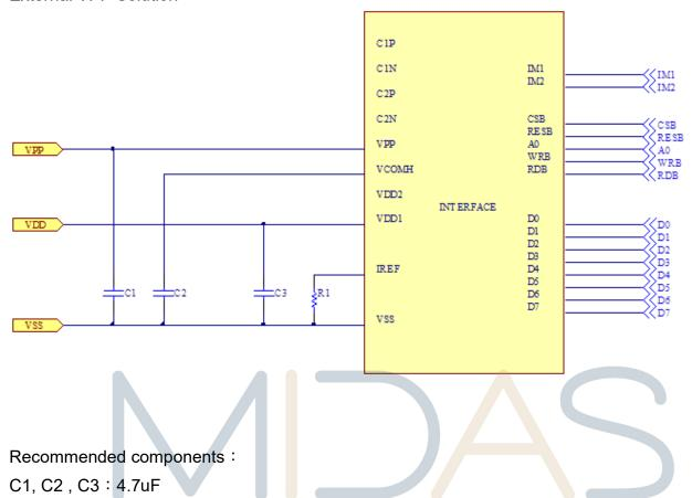
Bus Interface selection: (Must be set the IM[2:0], refer to item 3) 8-bits 6800 and 8080 parallel, 3 or 4-wire SPI, I2C
