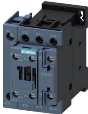
contactor AC-1, 50 A, 400 V / 40 °C, 4-pole, 24 V AC, 50 Hz, auxiliary contacts: 1 NO + 1 NC, screw terminal, size: S0
