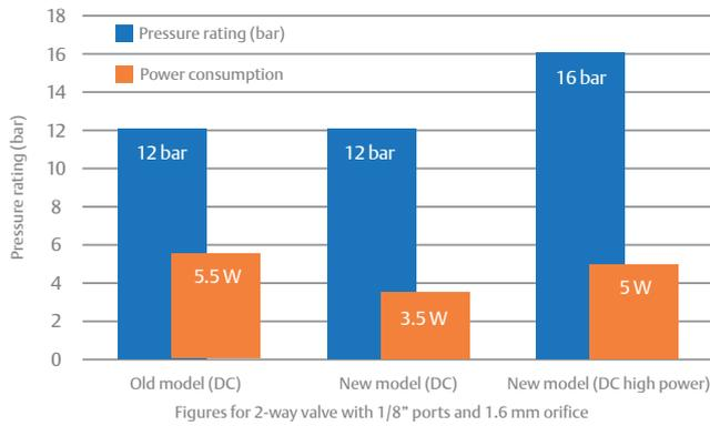
**Comparative pressure ratings** in a smaller valve typically results in increased power consumption, but the Series 256/356 actually reduces energy use by as much as 40%.
