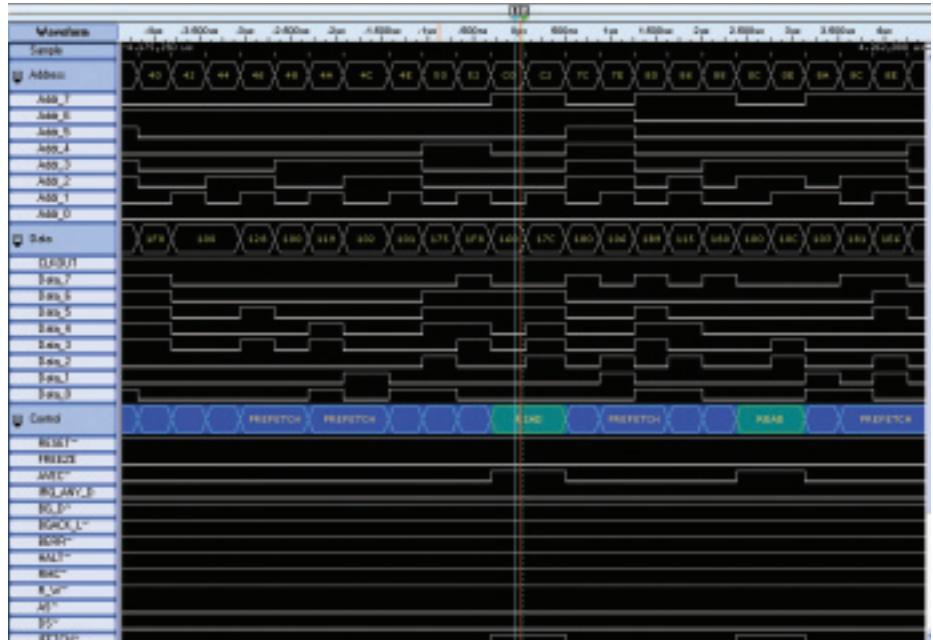
Figure 1. Logic Analyzer acquisition of a microcontroller's clock, address bus, data bus and control lines.
