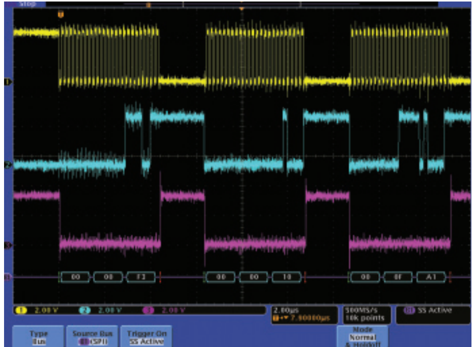
Figure 13. Correct synthesizer configuration messages.
