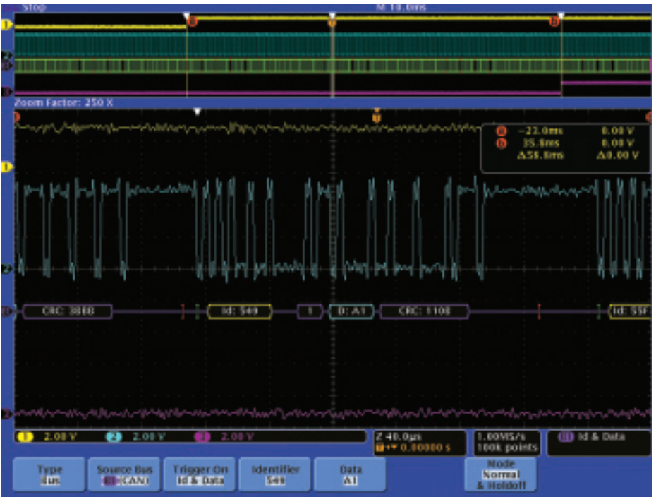
Figure 19. Triggering on specific identifier and Data on a CAN bus and decoding all messages in the acquisition.
