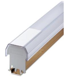
Cover profile, for covering terminal strips, snaps onto cover profile carrier AP 2-TU, can be marked with insert strip AP-ES. Cover profile carriers should be placed at the ends and at intervals of approx. 40 cm. Length: 1 m
