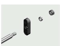
• Apply the screw locking agent contained in the set of wearing parts to the inside of the hex nut (the rear part of the piston rod on cylinders with through piston rod (S2 / S20)) and screw it onto the piston rod with the corresponding torque (see table).
