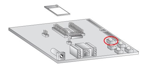
Press the reset button to reset the module. This is useful if you are having issues accessing the COM port. This also resets any parameters that were changed but not written into memory. Note that any changes written to the module are not changed when you reset it.
