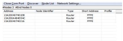
By selecting a particular node from the list, you can interact with it as if it were connected to the PC directly. Now you can Read, Write, and Restore parameters on the main XCTU window, and those changes occur over the air on the remote module selected in the Network window. Close the Network window when you have finished with remote configuration.
