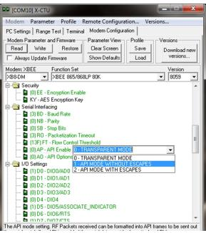
3. Set the base radio AP to 1:" Then in bullets beneath:
