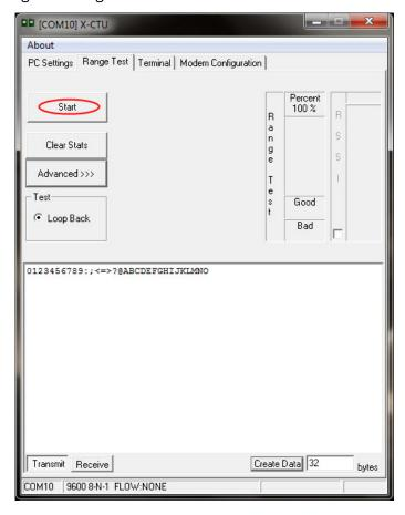
9. Monitor the link quality by reading the Percent section on the **Range Test** tab. This section displays the running percentage of good packets sent to the receiving radio and looped back to the base.
