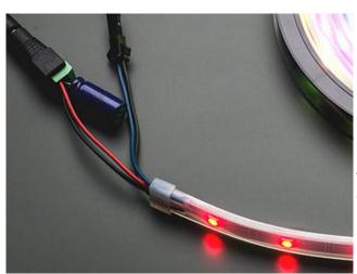
Before connecting a NeoPixel strip to ANY source of power, we very strongly recommend adding a large capacitor (1000  $\mu$ F, 6.3V or higher) across the + and – terminals. This prevents the initial onrush of current from damaging the pixels.
