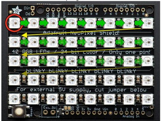
We refer to this layout as *row major* and *progressive*. *Row major* means the pixels are arranged in horizontal lines (the opposite, in vertical lines, is *column major*). *Progressive* means each row proceeds in the same direction. Some matrices will reverse direction on each row, as it can be easier to wire that way.
