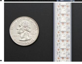
**NeoPixel Digital RGB LED Weatherproof Strip** is available in three different "densities": 30, 60 and 144 LEDs per meter, on a white or black backing strip.
