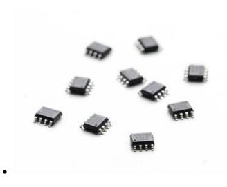
The NeoPixel driver logic is available separately (http://adafru.it/1378) from the LEDs, allowing power-users to create extremely customized designs...perhaps using other LED colors, or combined with power MOSFETs (http://adafru.it/355) to control high-current LEDs or "analog" RGB LED strips (http://adafru.it/ICy) using the NeoPixel protocol.
