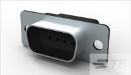
TE Part #205204-8 HDP-20,PLUG,SIZE 1, 9 POSN
