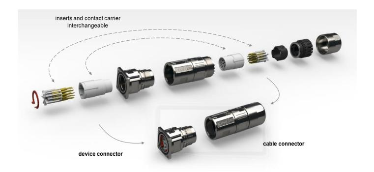
M17 circular connectors offer a high degree of flexibility and versatility in a compact and robust housing. With their high contact density and large current carrying capacity in a small installation space, the M17 circular connectors are ideal for use in systems with limited space. The har-lock fast locking system is pluggable with the M17 fast locking systems Speedtec and ONECLICK.
