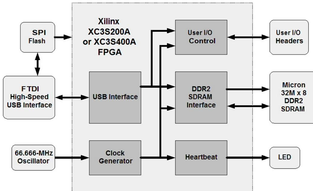
It contains a USB Interface Block, a User I/O Block, a DDR2 SDRAM interface, a Heartbeat Pulse Generator and a Clock Generator. The SPI Flash is used to store the design's FPGA configuration file.
