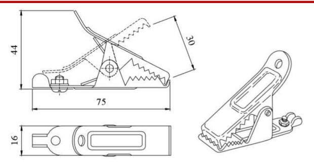
PVC INSULATED BOOT AVAILABLE IN RED 310-0500 OR BLACK 310-0100 OPERATING TEMPERATURE WITH BOOT FITTED -20 TO +60°C
