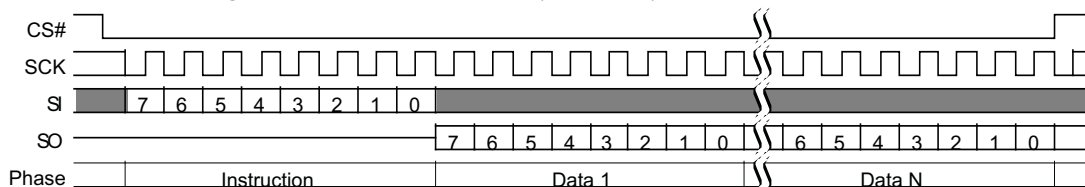
Figure 48. Read Identification (RDID 9Fh) Command Sequence
