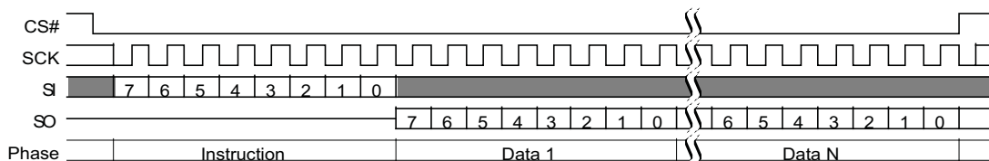
Figure 117. Password Read (PASSRD E7h) Command Sequence
