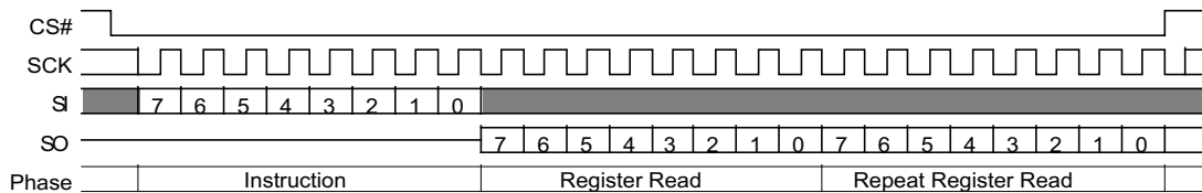
Figure 54. Read Bank Register (BRRD 16h) Command
