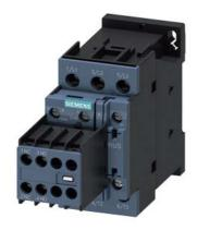
power contactor, AC-3e/AC-3, 32 A, 15 kW / 400 V, 3-pole, 230 V AC, 50 Hz, auxiliary contacts: 2 NO + 2 NC, screw terminal, size: S0, removable auxiliary switch
