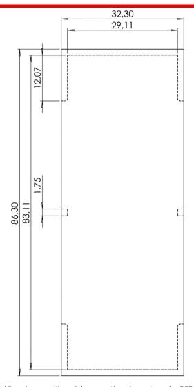
Dashed line shows outline of the mounting elements under PCB board All dimensions are given within +/-0,25mm tolerance
