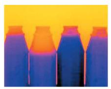
Detecting liquid levels in visually opaque bottles.
