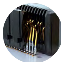
Differential pair for increased speed (HSEC8-DP)
