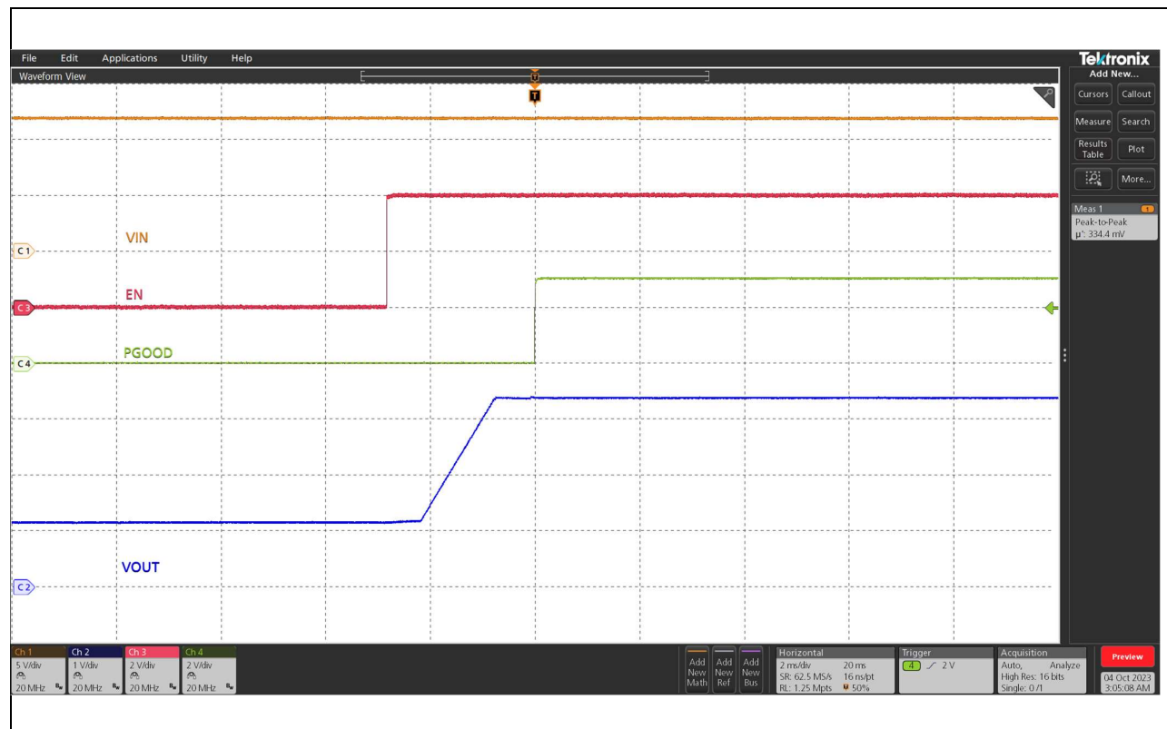
Figure 11 Pre-bias Start up at 0 A Load, (Ch1: Vin, Ch2: Vout, Ch4:PGood ,Ch3:Enable)
