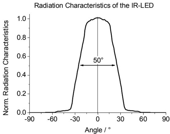
Fig. 11: Radiation characteristics of the proximity sensor LED.
