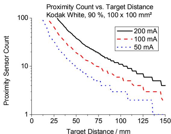
Fig. 8: Proximity sensor signal vs. target distance and LED drive current (reflector: Kodak White, 90 %, 100 x 100 mm<sup>2</sup>).
