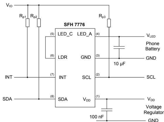
Fig. 20: Recommended implementation into a mobile phone environment.
