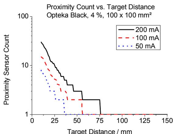
Fig. 10: Proximity sensor signal vs. target distance and LED drive current (reflector: Opteka Black, 4 %, 100 x 100 mm<sup>2</sup>).
