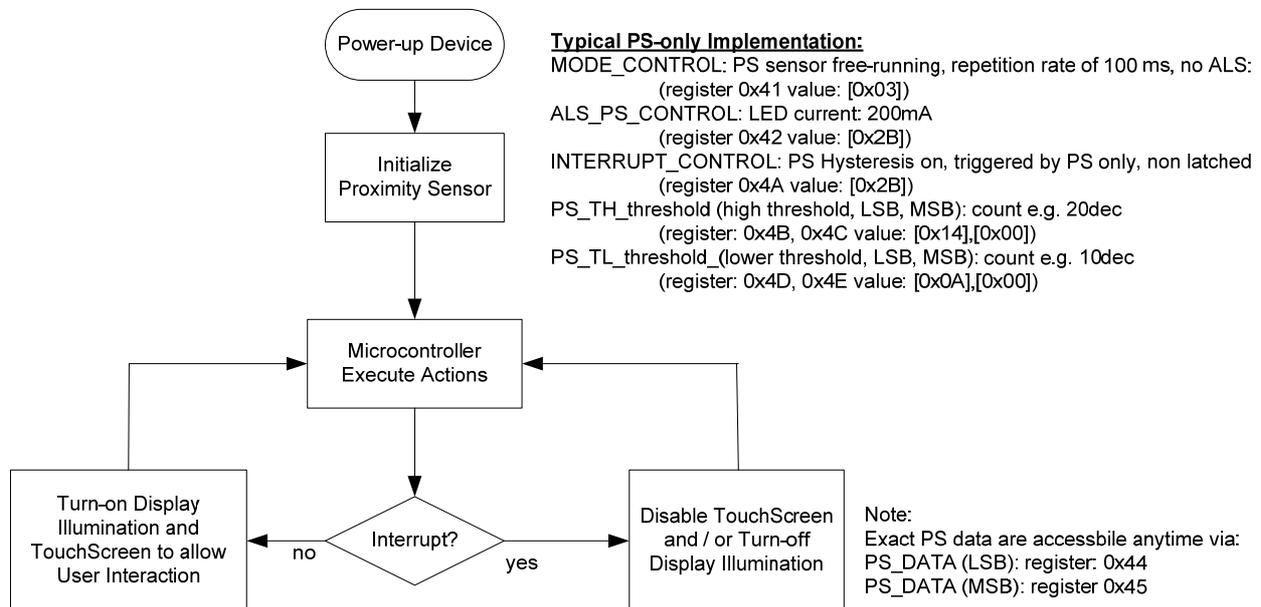
Fig. 22: Flowchart for a microcontroller based proximity sensing example.
