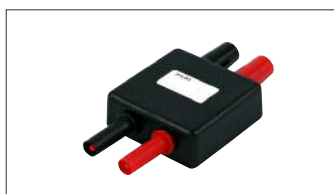
989006000 : 1 ohm shunt, 0.1%, 0.5A max
