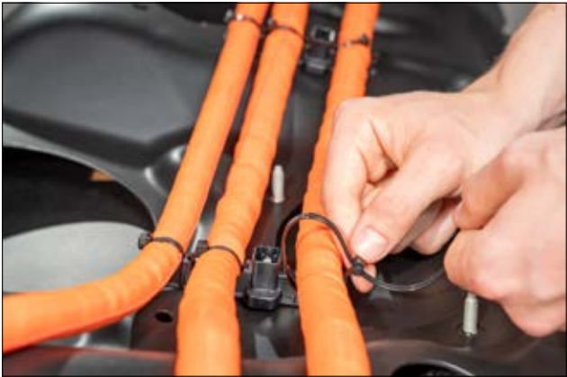
Fixing tie for cable bundles/for stud, outside serrated, 8.0-26.0mm
