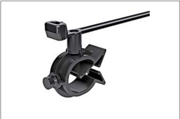
Cable tie combined with a 360° rotatable open clip that allows compensating movements and can be retrofitted to an already installed cable harness.
