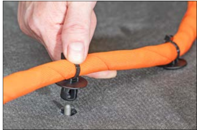
Pre-assembled two-piece fastening tie with weld stud foot — enables quick, secure mounting on 5 and 6 mm bolts with insertion forces below 30 N.
