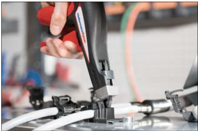
Tension tab can be used to ensure specific tension.
