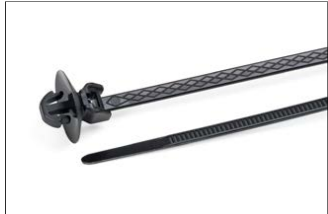
T30SOS-AS-SFT6.5x4E, 1 piece fixing tie with AntiSlip engraving for a round hole 6.5 mm or a square hole 6.5x4 mm.
