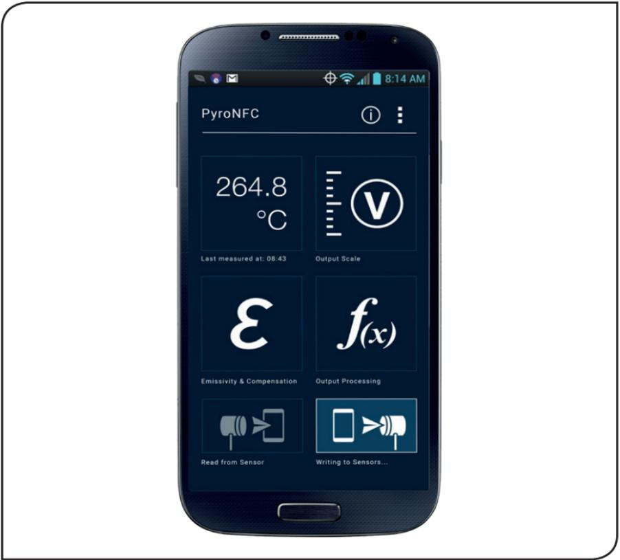
Touch the NFC device against the back of the sensor to read the measured temperature. The reading updates continuously while the phone is touching the sensor.
