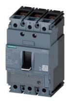
circuit breaker 3VA1 IEC frame 160 breaking capacity class M Icu=55kA @ 415V 3-pole, starter protection TM120M, AM, In=50A without overload protection short-circuit protection Ii=7...16 x In nut keeper kit
