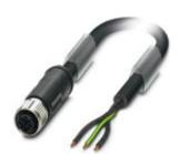
Power cable, 3-position, PVC, black, free cable end, on Socket straight M12 SPEEDCON, S-coded, Cable length: 5 m, For AC current up to 16 A/230 V
