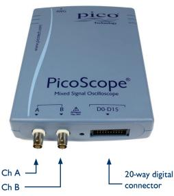
The front panel of the PicoScope 2205 MSO has two BNC analog input channels and a 20-way connector with 16 digital inputs.
