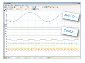
The PicoScope 2205 MSO is a full-featured oscilloscope. A function generator and arbitrary waveform generator are built-in and include a sweep function. It also offers mask limit testing, math and reference channels, advanced digital triggering, serial decoding, automatic measurements and color persistence display.
