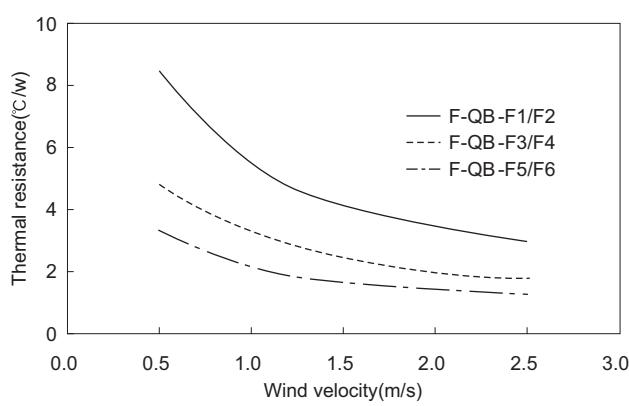
Fig.7 Thermal resistance of heat sink(Forced air)
