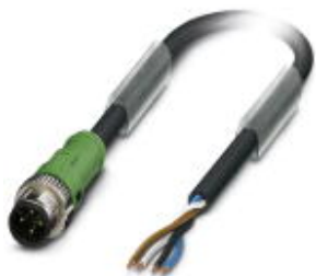
Sensor/Actuator cable, 4-position, PUR, black-gray RAL 7021, Plug straight M12 SPEEDCON, A-coded, on free cable end, Cable length: 2 m
