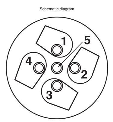
Cable connection side M12 (screw connection)
