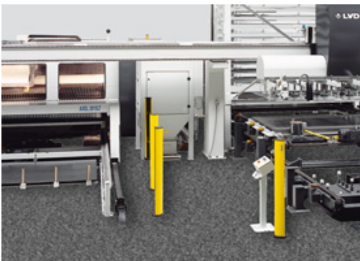
Access protection with a multiple light beam safety device (type 4) for a laser cutting system with automatic sheet metal store.
