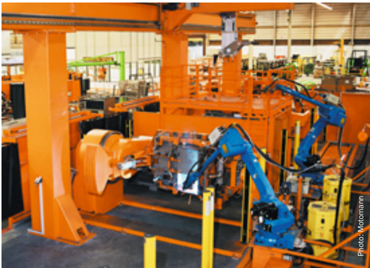
Efficient work without danger — robot protection with type 4 multiple light beam safety devices Active/Passive.
