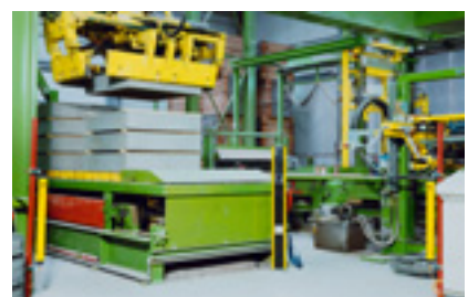
Two-side access protection system with M2000 and mirror column.
