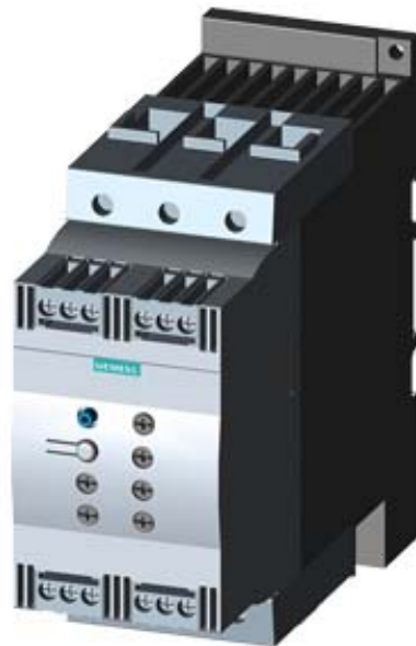
SIRIUS SOFT STARTER, S3, 80A, 45KW/400V, 40 DEGR., AC 200-480V, AC/DC 110-230V, SCREW TERMINALS
