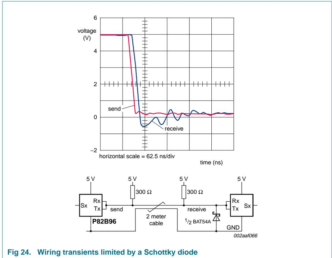
**Fig 24. Wiring transients limited by a Schottky diode**
