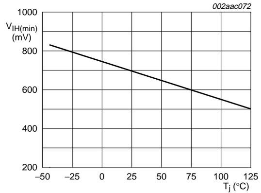
$V_{IH(min)}$  at  $S_x$  changes over temperature range
