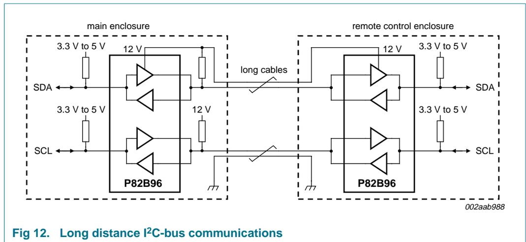
**Fig 12. Long distance I<sup>2</sup>C-bus communications**
