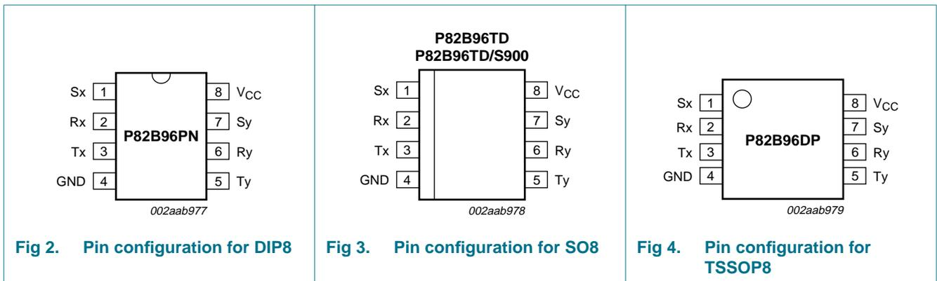
Fig 2. Pin configuration for DIP8
