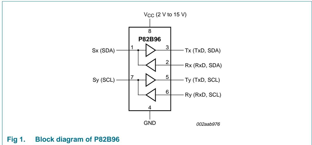
Fig 1. Block diagram of P82B96
