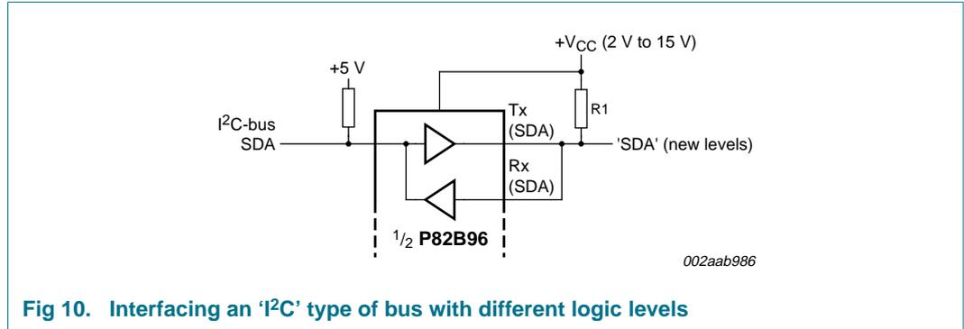
**Fig 10. Interfacing an 'I<sup>2</sup>C' type of bus with different logic levels**
