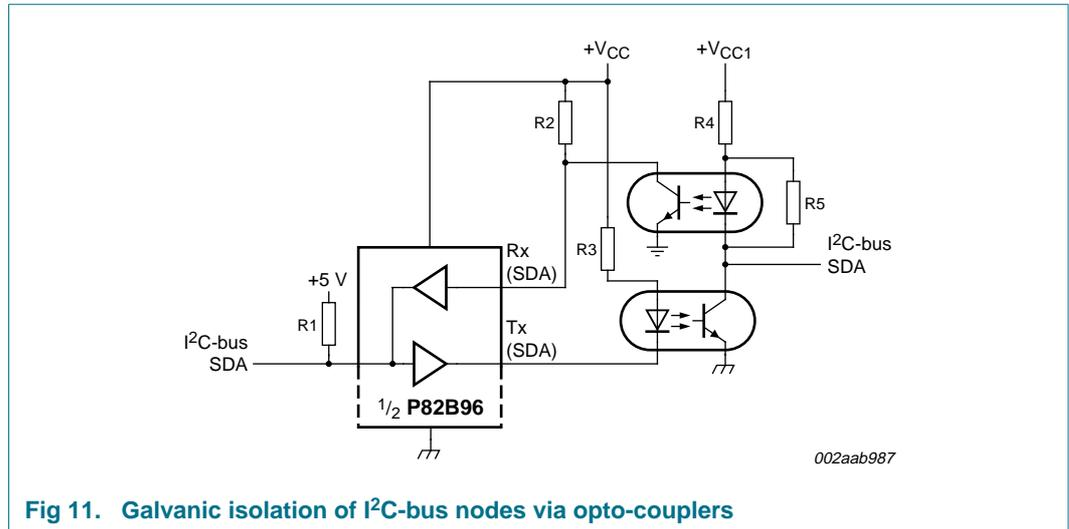
**Fig 11. Galvanic isolation of I<sup>2</sup>C-bus nodes via opto-couplers**
