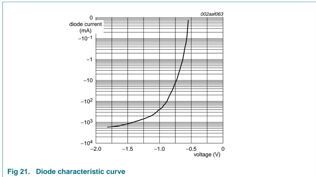
**Fig 21. Diode characteristic curve**
