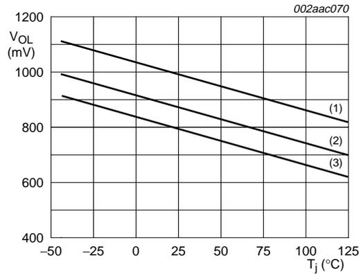
$V_{OL}$  at  $S_x$  typical and limits over temperature
