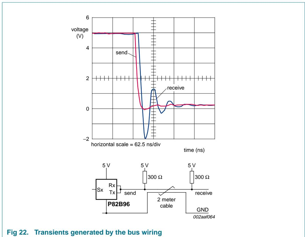
Fig 22. Transients generated by the bus wiring
