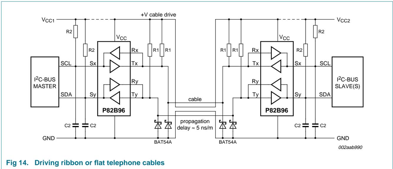
Fig 14. Driving ribbon or flat telephone cables
