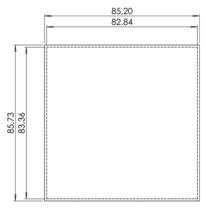
Dashed line shows outline of the mounting elements under PCB board All dimensions are given within +/-0,25mm tolerance
