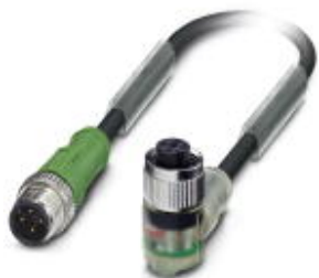
Sensor/Actuator cable, 4-position, PUR halogen-free, black-gray RAL 7021, Plug straight M12, A-coded, on Socket angled M12, A-coded, with 3 LEDs, Cable length: 3 m
