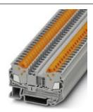
Feed-through terminal block, Connection method: Quick connection, Cross section: 0.5 mm² - 2.5 mm², AWG: 20 - 14, Width: 6.2 mm, Color: gray, Mounting type: NS 35/7,5, NS 35/15
