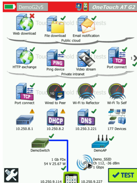
Figure 9. Group tests by hosting location – local, intranet, internet
