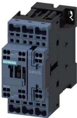
power contactor, AC-3e/AC-3, 38 A, 18.5 kW / 400 V, 3-pole, 200-280 V AC/DC, 50/60 Hz, with integrated varistor, auxiliary contacts: 1 NO + 1 NC, spring-loaded terminal, size: S0
