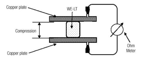
Fig. 4: Test setup surface resistance WE-LT vs. compression
