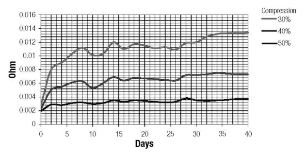
Fig. 5: Long-term run surface resistance vs. compression
