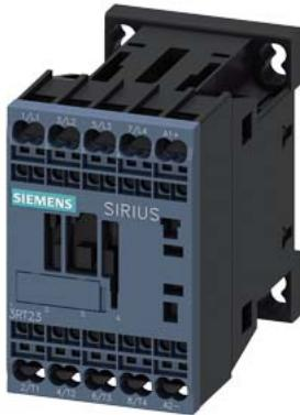
Schütz AC-1, 22 A, 400 V / 40 °C, 4-polig, DC 24 V, Federzuganschluss,
