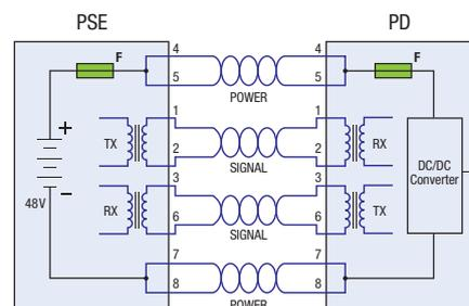
**Fig. 1: Standard configuration of PoE and PoE+: two separate conductor pairs for power and signals. Chip fuses (F) protect the electronics simply and securely from overcurrents (Source: SCHURTER AG)**
