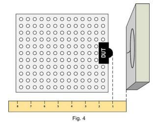
The DUT was positioned a known distance from the RF antenna prior to transmission of the RF test pattern.
