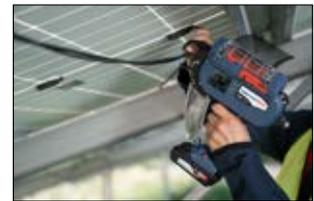
Fast and flexible cable bundling tool CPK hybrid for portable use on solar plants anywhere.
