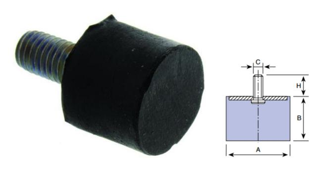
These buffers are made with a rubber compound permitting major deformations under impact with notable absorptions of energy. They can be made with high-damping rubber to order, however, absorption of energy in high damped compound buffers is performed with reduced rebound movement but with slightly higher transfer levels of stress to the structure.
