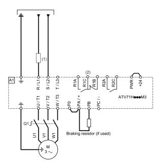
(1)Line reactor, if used (compulsory for ATV71H U40M3 to U75M3 drives) (2)Fault relay contacts, for remote signaling of drive status
