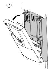
$\fbox{7}$  Replace the control front panel over the option card (same procedure as for installing the option card, see  $\fbox{5}$  and 6)
