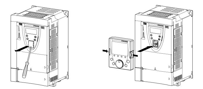
The graphic display terminal can be connected or disconnected with the power on. Before disconnecting it, drive control via the display terminal must be disabled (refer to the programming manual).
