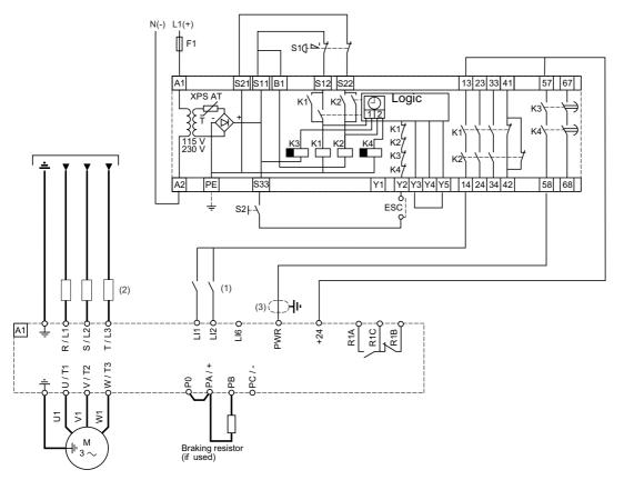
(1) In this example, the logic inputs LIe are wired as "Source" but can be wired as "Int Sink" or "Ext Sink".
