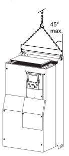
ALTIVAR 71 drives up to ratings ATV71HD15M3X and ATV71HD18N4 can be removed from their packaging and installed without a handling device.
