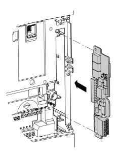
If an I/O or communication option card or a "Controller Inside" programmable card has already been installed, remove it so you can access the slot for the encoder interface card.
