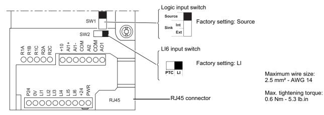
Note: The ATV71 is supplied with a link between the PWR and +24 terminals.
