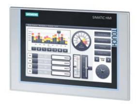
SIMATIC HMI TP900 COMFORT, COMFORT PANEL, FUNZIONALITA' TOUCH, DISPLAY TFT WIDESCREEN DA 9", 16 MILIONI DI COLORI, INTERFACCIA PROFINET, INTERFACCIA MPI/PROFIBUS DP, MEMORIA DI PROGETTAZIONE 12 MB, WINDOWS CE 6.0, PROGETTABILE DA WINCC COMFORT V11
