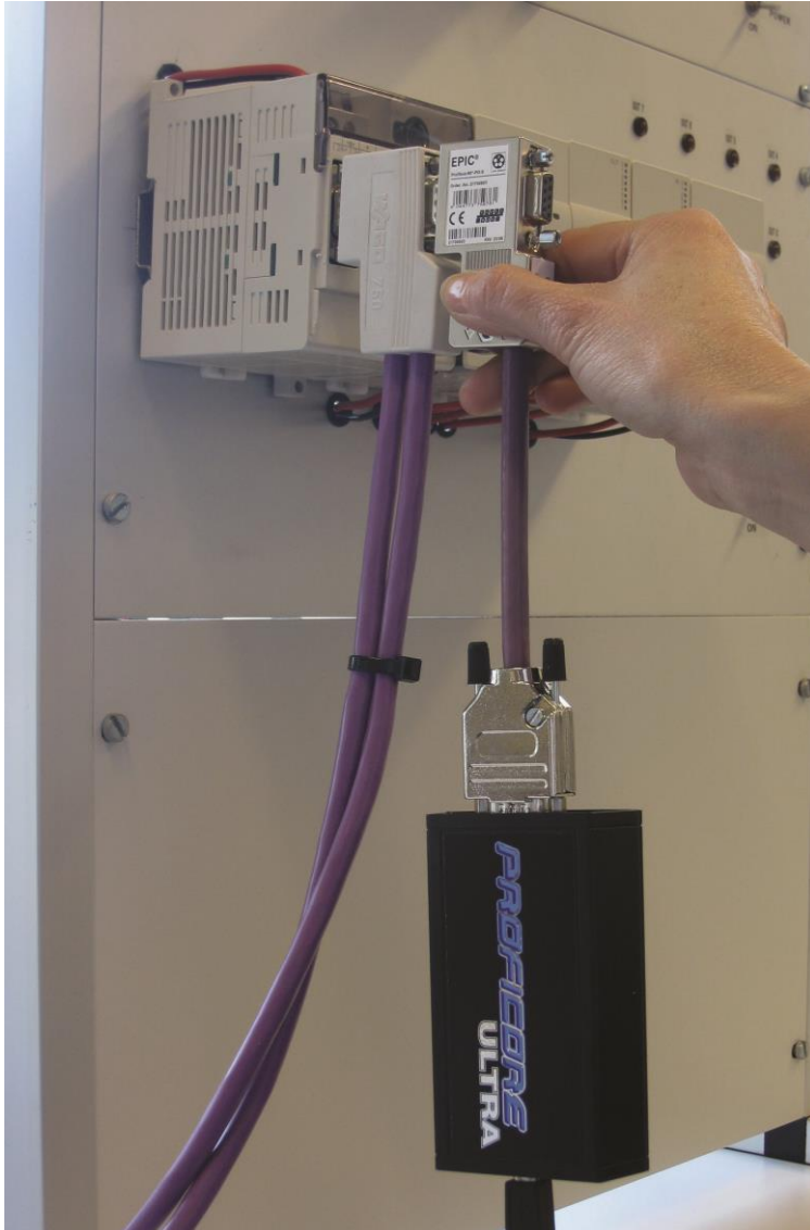
Fig. 10 - Attaching the ProfiCore to a DP installation
