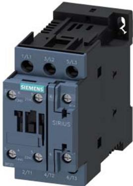
power contactor, AC-3e/AC-3, 38 A, 18.5 kW / 400 V, 3-pole, 95-130 V AC/DC, 50/60 Hz, with integrated varistor, auxiliary contacts: 1 NO + 1 NC, screw terminal, size: S0
