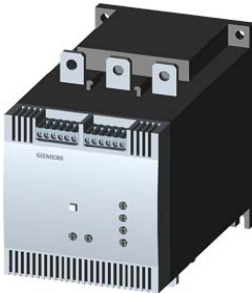
SIRIUS SOFT STARTER, S12, 280 A, 160 KW/400 V, 40 DEG., 200-460 V AC, 230 V AC, SCREW TERMINALS
