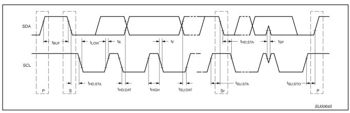
Figure 13. Definition of timing on the I<sup>2</sup>C-bus
