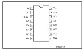
Figure 1. Pin configuration
