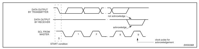
Figure 9. Acknowledgement on the I<sup>2</sup>C-bus
