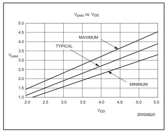
Figure 5.  $V_{pass}$  voltage vs.  $V_{DD}$
