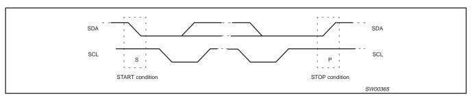
Figure 7. Definition of start and stop conditions
