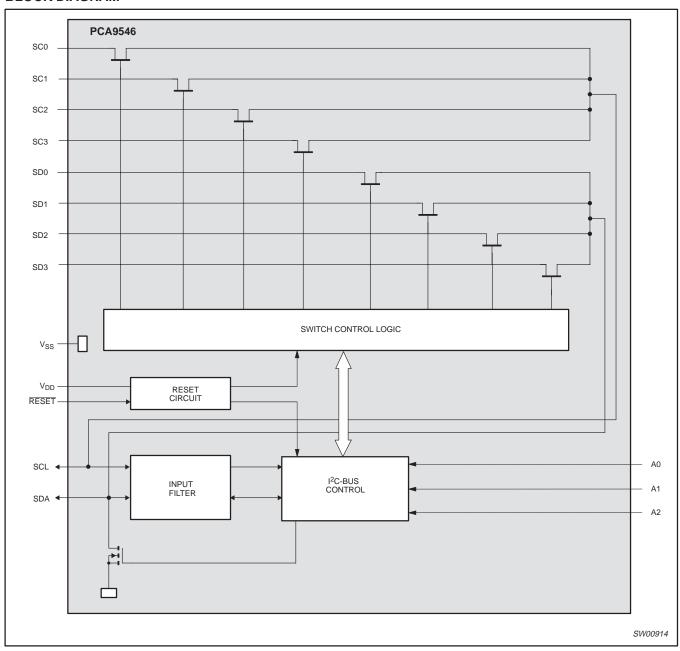
Figure 2. Block diagram
