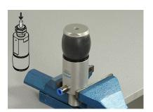
Carefully cut apart the worn bellows in longitudinal direction using a sharp knife (cutter knife, utility knife).
